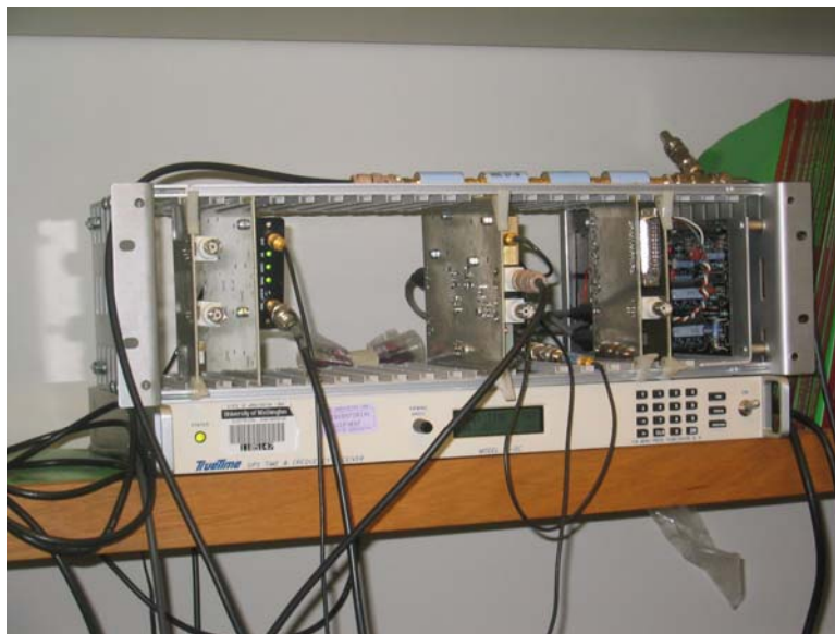
Figure 12: Manastash Ridge Radar receiver, showing the simplicity of the digital receiver and GPS synchronisation hardware.
